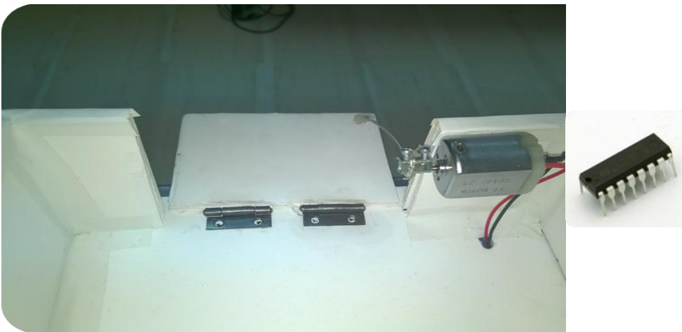
Fig. 5. DC motor & H-Bridge
