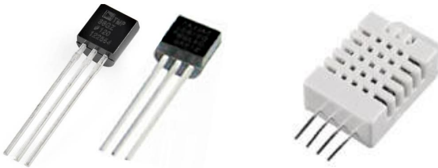
Fig. 8. Temperature sensors TMP36GZ / TMLM35 and Humidity sensor RHT03
