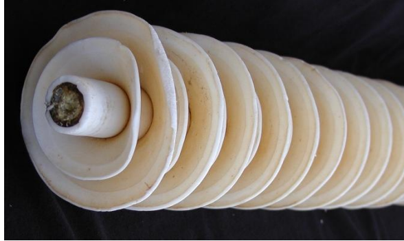
Fig. 3. PTFE insulator destroyed due to the action of brittle fracture
