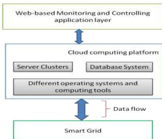
Fig 3 Cloud-based SCADA configuration
