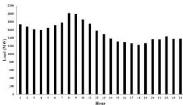
Fig. 7 Illustration of the electricity load pattern during the studied day
