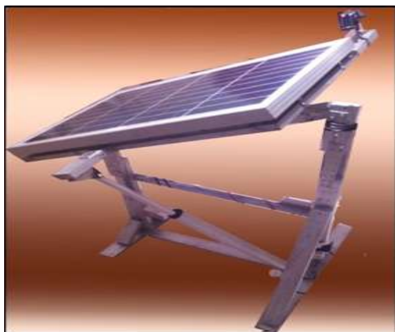
Fig. 3 Single axis tracking system
