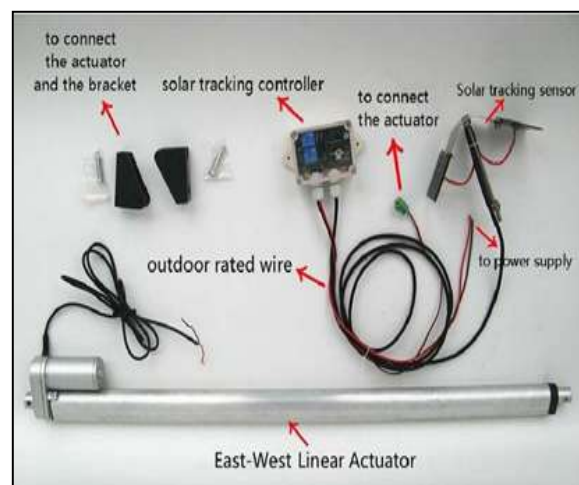
Fig. 6 Solar Tracking sensor, controller and actuator
